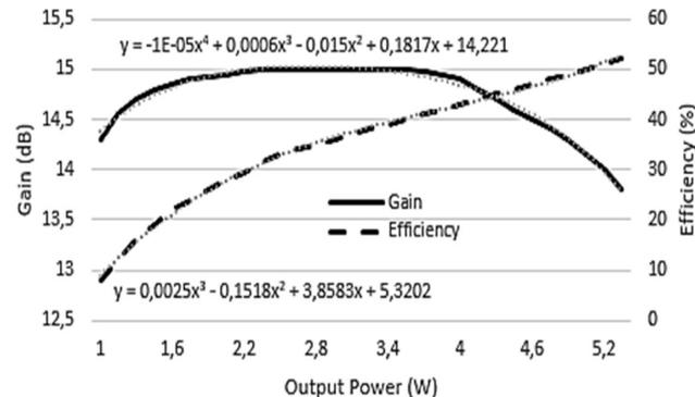
NPTB00004A: a GaN amplifier manufactured by MACOM, with the following characteristics:
