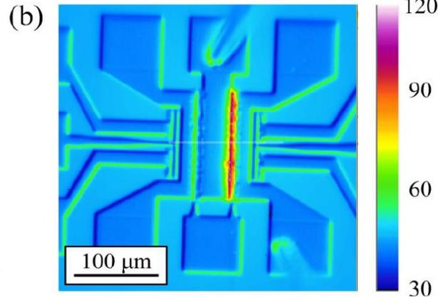
(a) Blackbody infrared spectrum and (b) Sample infrared temperature ( $^{\circ}\text{C}$ ) map of GaN HEMT
