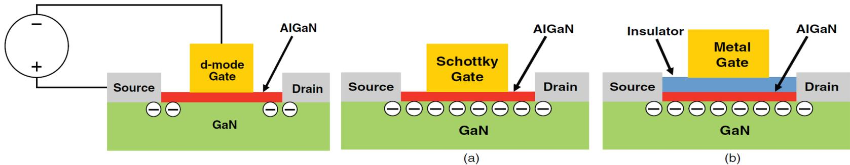
Cross section of a basic depletion-mode GaN HEMT with (a) Schottky gate, or (b) Insulating gate. In power conversion applications, d-mode devices are inconvenient because, at the startup of a power converter, a negative bias must first be applied to the power devices (such as GaAs and InP microwave devices). If this negative bias is not applied first, a short circuit will result between drain and source.
