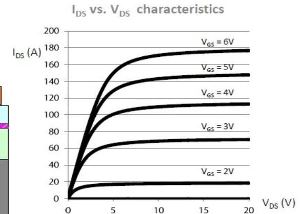
A GaN MOSFET power switch is built on a silicon substrate (Si or SiC), with a lateral two-dimensional electron gas (2DEG) channel formed on a AlGaN/GaN hetero-epitaxy structure that provides very high charge density and mobility; the enhancement-mode GaN device does not conduct when the gate drive is at zero but does conduct when the gate drive exceeds the threshold.
