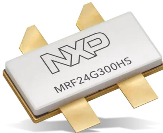
The new MRF24G300HS is a 50V GaN-HEMT with more or less similar characteristics but it has an efficiency of 73% at the same frequency and it can tolerate 20:1 of VSWR at all phase angles. Internally there are two sections so this device can be used in a single-ended or push-pull configuration.
