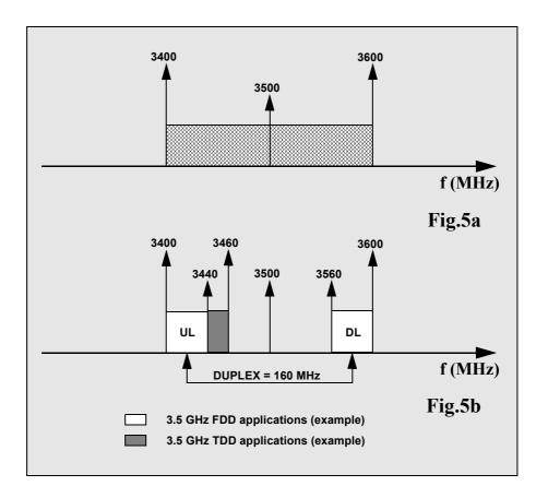
In any case, this will be one of the most critical point for FDD terminals implementation at 3.5 GHz even though the duplex space will be widen in the future (3.4 - 3.8 GHz is planned in Canada) [14].
