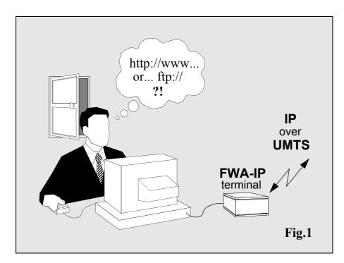
An FWA-IP terminal can be represented by a single box, as shown in fig.1, but it could be implemented by one, two or more different phisical boxes, connected together by cables. Obviously, one box solution seems to be the right choice, because surely it has lower costs and it will be easier to install but, on the other hand, it has some drawbacks, which are described below.
