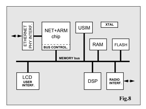
Proposal N.3 seems to be the best choice because the Net+Arm is designed to operate with Network protocols, so it is possible to develop the product better, faster and at lower cost. PowerPC405 has been designed to work on ethernet as well, but it is not available yet.
