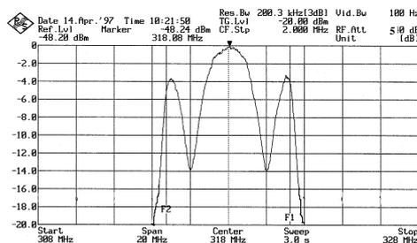
Fig. 4.35 Fading spectrum
