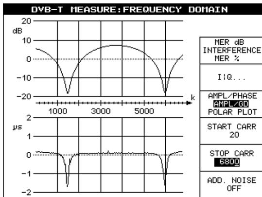
Fig. 4.50 Linear distortion (amplitude and phase) due to fading in transmission channel (with carrier number  $k$  plotted along abscissa)
