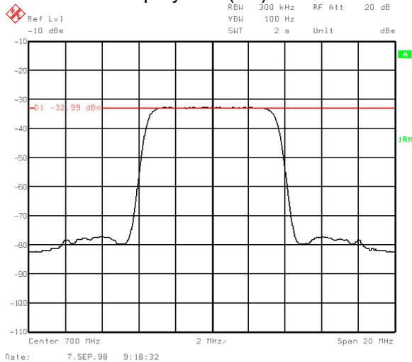
Fig. 6a PRBS spectrum: level marked with display line, 10 dB/div
