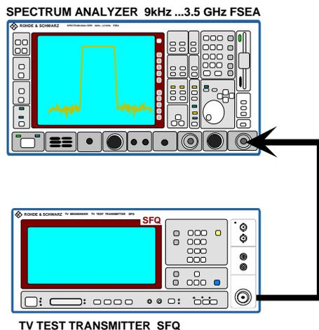
Fig. 4 Block diagram of SFQ and FSE
