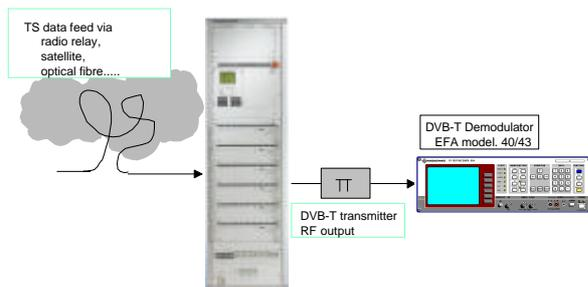
Longterm measurements with Test Receiver EFA model 40/43
