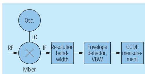
tion is eliminated from the signal; only the “envelope” signal is used (FIG 2). The measured values of a pure CW signal always have the same amplitude; it has thus a crest factor of 0 dB. In the case of IF and video filtering, it must be ensured that the resolution bandwidth (RBW) and the video bandwidth (VBW) do not distort the signal:
