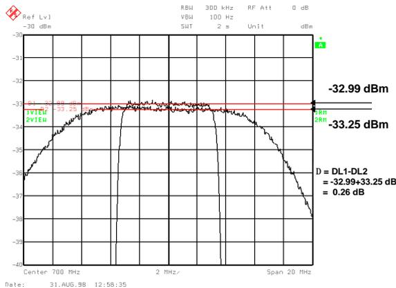
Fig. 9 Measurement of deviation from selected C/N value
