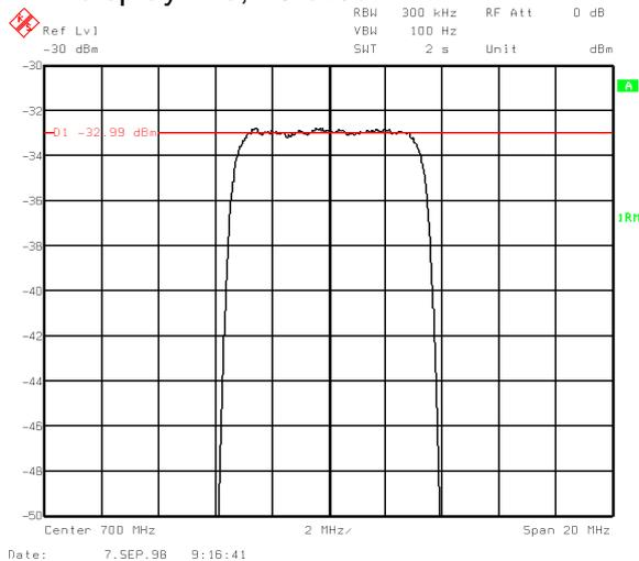
Fig. 6b PRBS spectrum: level marked with display line, 1 dB/div
