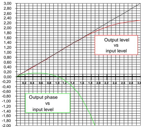
Fig. 4.27 Amplifier characteristic
