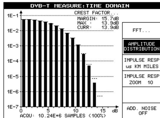
Fig. 4.32 Crest factor measurement with DVB-T Test Receiver EFA model 40 or 43
