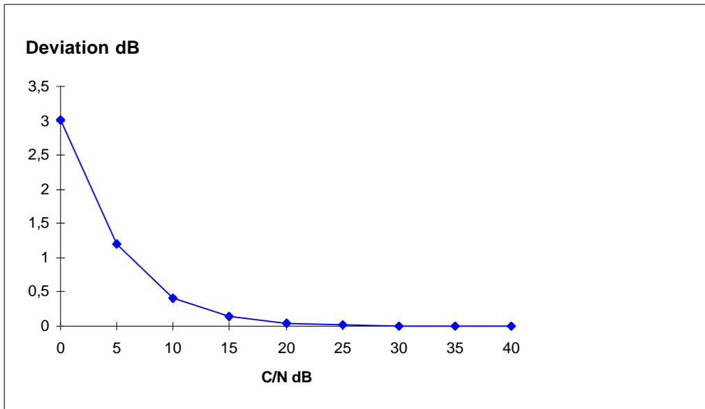
The above diagram shows that the effect of superimposed noise concerning the output power is negligible from a C/N value of >23 dB. For values <20 dB, BER measurement is error-prone already for 64 or 256QAM signals.
