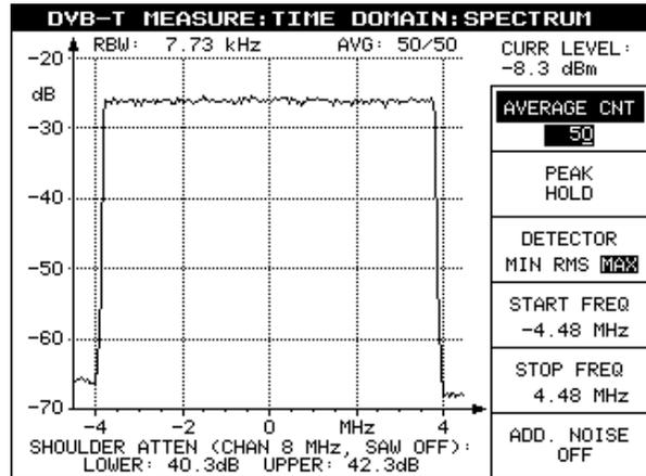
Fig. 4.25 Shoulder distance of COFDM signal
