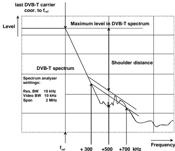
Fig. 4.26 Measurement of shoulder distance to ETR290
