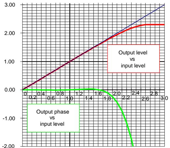
Fig. 4.29 Typical gain and phase characteristics of corrected amplifier
