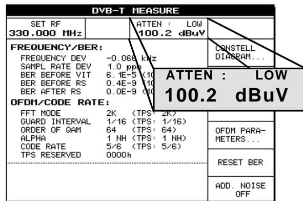
Fig. 4.34 Measurement menu of Test Receiver EFA model 40 or 43
