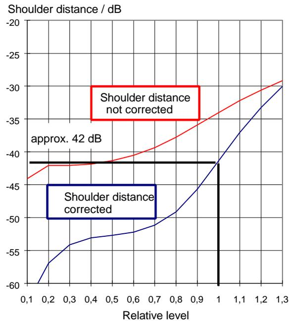
Fig. 4.30 Shoulder distance obtained with corrected/non-corrected amplifier
