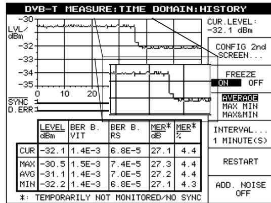
Fig. 4.39 Histogram generated by Test Receiver EFA model 40/43
