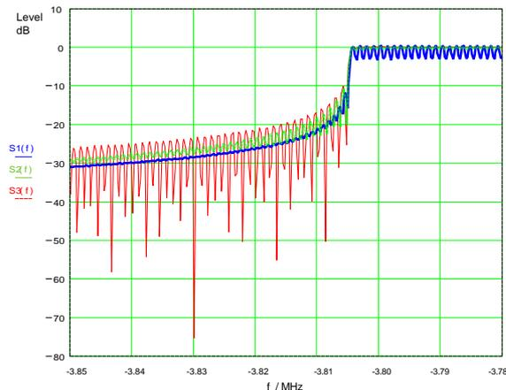
Fig. 4.17 Detail of spectrum with different guard intervals:
