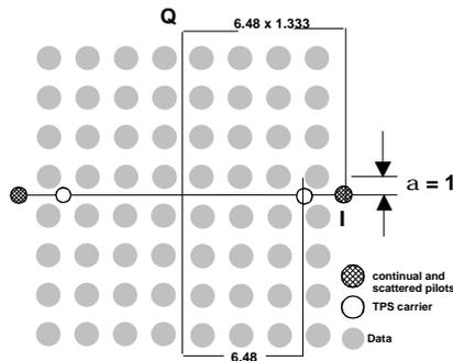
Fig. 4.9 Constellation diagram with pilots and TPS carriers, non-hierarchical
