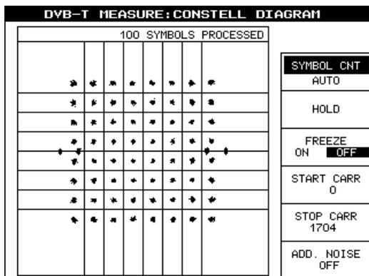
Fig. 4.54 Constellation diagram for 64QAM, 2k mode
