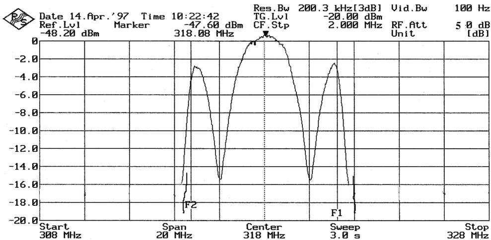
The above diagrams show that the results obtained with NRV and EFA virtually coincide. This demonstrates the high precision of power measurements made with EFA in a QAM-modulated channel also under critical conditions.
