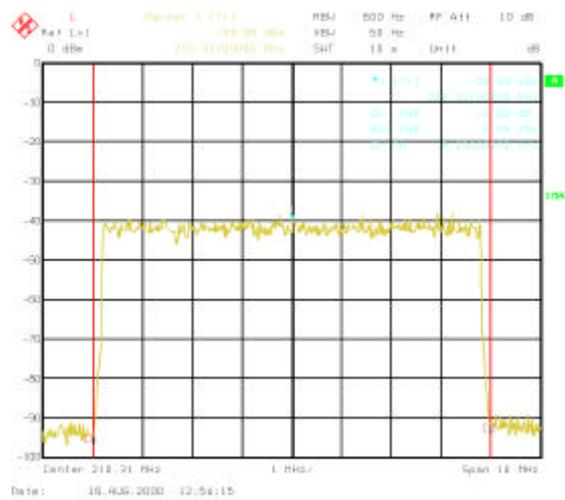
Fig. 4.33 Power measurement with frequency cursor
