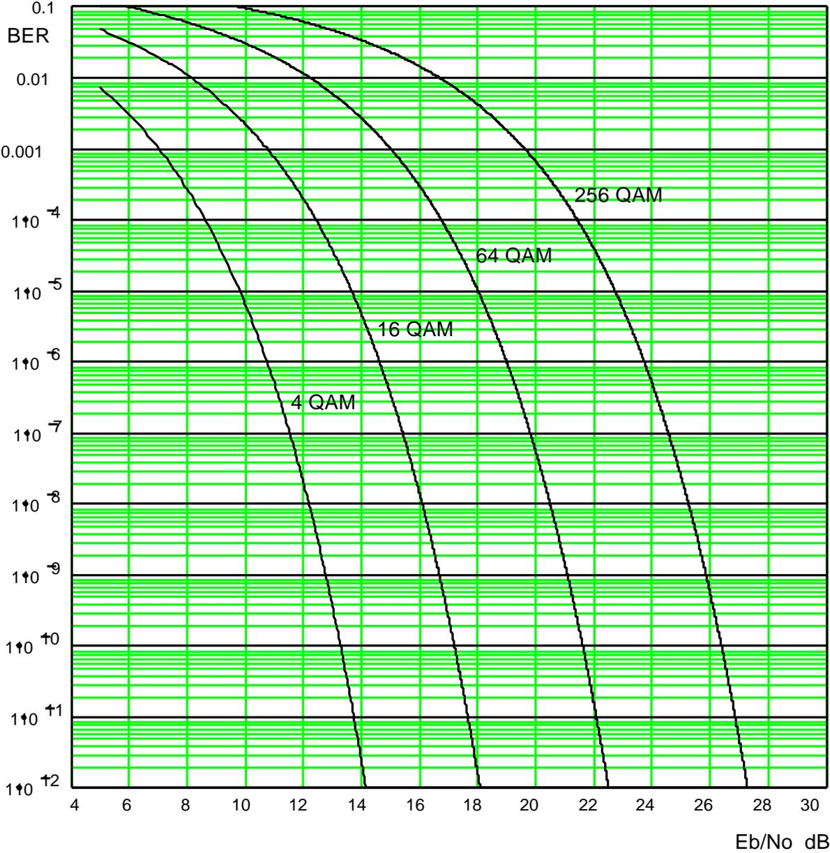
Fig. 12 BER as a function of Eb/No
