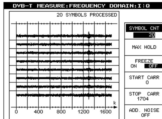
Fig. 4.58 I/Q analysis of 2k COFDM signal
