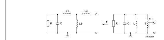
Fig.3-38 Norton transformation at transistor output.
