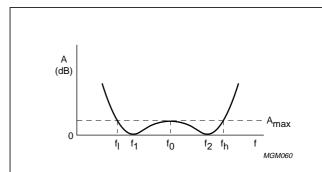
Fig.3-31 Pass-band characteristic of the two-section matching circuit of Fig.3-30.
