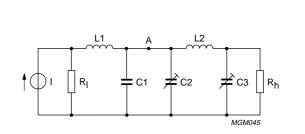
Fig.3-16 Impedance matching circuit using only parallel capacitors.
