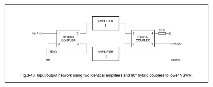
This sort of hybrid coupler with a full octave bandwidth and continuous power handling of 200 W is available from Anaren, USA.
