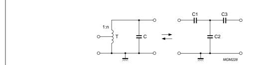
Fig.3-39 Alternative transformation at 50  $\Omega$  load side.
