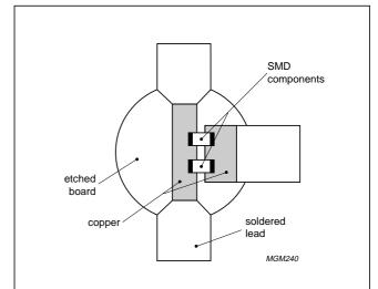
Fig.3-52 Dummy load made using printed-circuit board and SMD components. Though the dimensions are not critical, it is convenient to mimic those of a transistor to form a drop-in transistor replacement during alignment.
