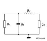
Fig.3-20 Output capacitance compensation using one element.
