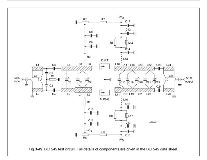
In the VHF and UHF ranges, another kind of balun is often used. Take, for example, the 500 MHz test circuit of the BLF545 (Fig.3-49). Although this is a narrow-band circuit, the balun used is a wideband type with a bandwidth of approximately one octave. Note that owing to the operating frequency, extensive use is made of striplines.
