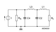
Fig.3-30 Two-section matching network for the upper VHF range.
