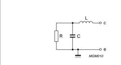
Fig.3-36 Equivalent circuit of the output of a transistor without internal output matching.
