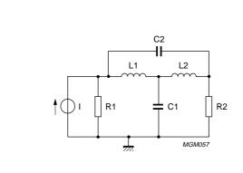
Fig.3-28 Second example of an improved compensation circuit for the lower VHF range.
