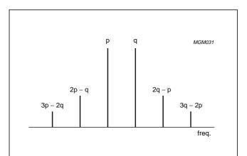
Fig.3-1 Position of the main intermodulation distortion products in the 2-tone test where p and g are the input tones.
