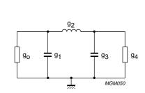
Fig.3-21 Output capacitance compensation using two elements.
