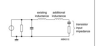
Fig.3-8 Adding a series inductance to the input matching circuit A of Fig.3-7 to compensate for the capacitive part of a transistor's input impedance.
