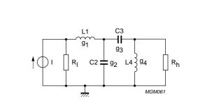
Fig.3-32 Two-section matching network using two L-sections.
