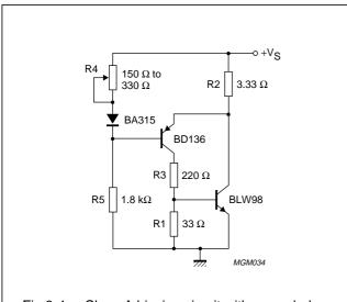
Fig.3-4 Class-A biasing circuit with grounded emitter for maximum power gain.
