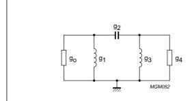
Fig.3-23 Compensation of an RF choke and impedance transformer.
