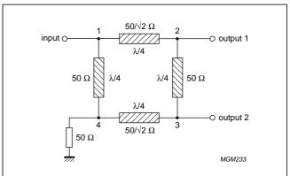
Fig.3-44 90° hybrid coupler based on striplines.
