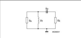
Fig.3-22 Compensation of an RF choke.
