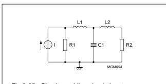
Fig.3-25 Circuit providing simple input compensation of a MOS transistor.
