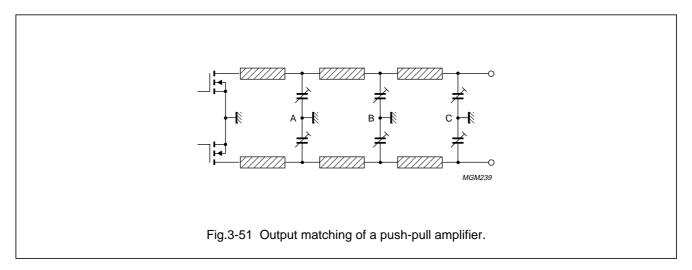
The last step is to choose the reactances of the capacitors  $C_{23}$  and  $C_{24}$  which have to be equal to the series-equivalent inductive reactances.
