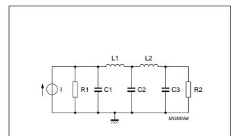
Fig.3-27 Example of an improved compensation circuit for the lower VHF range.
