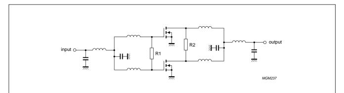
Fig.3-48 Two-transistor power amplifer with matching sections. This arrangement is also suitable for bipolar transistors.
