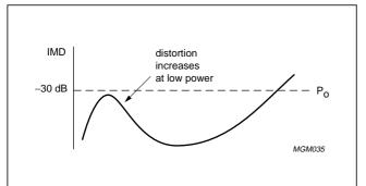
Fig.3-5 Intermodulation distortion as a function of output power for a class-AB amplifier.
