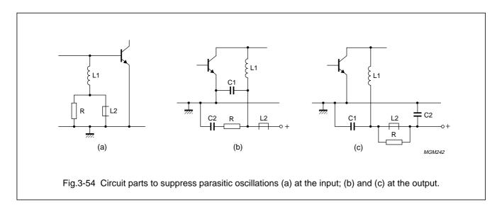
Also possible is a parametric oscillation known as conversion oscillation. This can happen when the collector or drain circuit contains two resonant circuits where the sum of the resonant frequencies equals the frequency of operation. The lower one is then formed by the RF choke and the total effective parallel capacitance while the other is the slightly detuned output matching circuit. This detuning can arise during tuning or by a small antenna mismatch.
