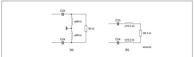
Fig.3-50 (a) Modified output baluns using 1/8  $\lambda$  stripline; (b) Transformed circuit of (a) using the parallel-to-series transformation described in Section 3.2.1.1.
