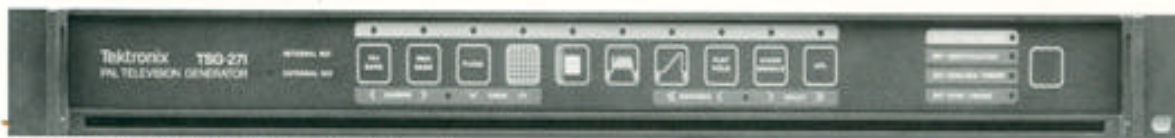
Figure 1. Tektronix TSG-271 PAL Test Signal Generator.
