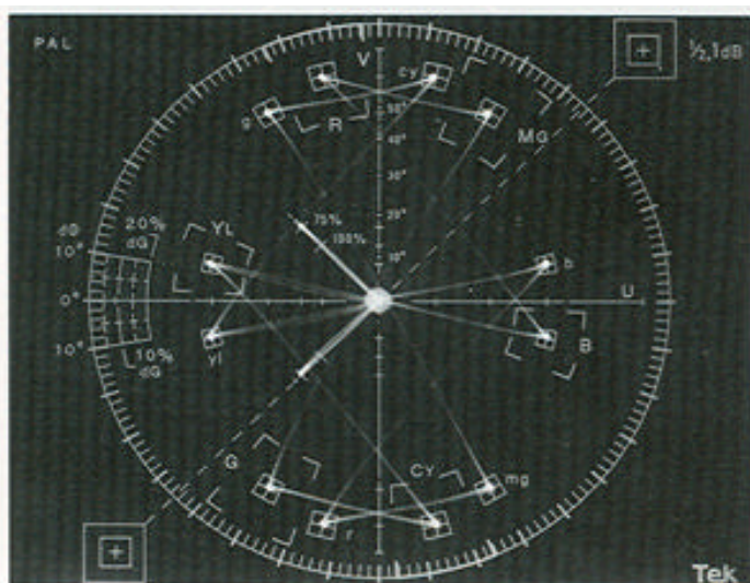
Figure 3. A vectorscope display of Colour Bars.
