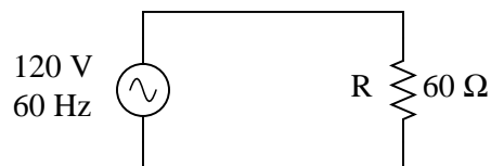
Figure 11.1: Ac source drives a purely resistive load.
