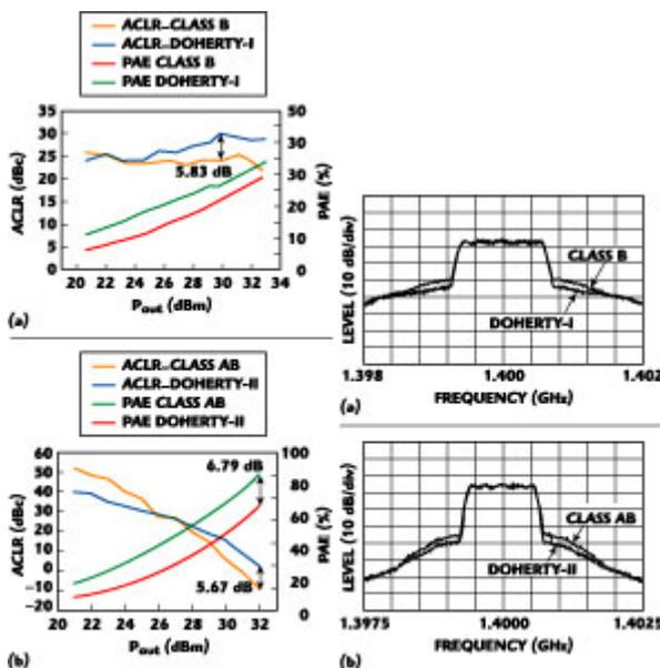
**Fig. 11** ACLR at 885 KHz offset and the PAE vs. output power for a CDMA signal for the (a) Doherty-I and class B amplifiers and (b) Doherty-II and class AB amplifiers.
