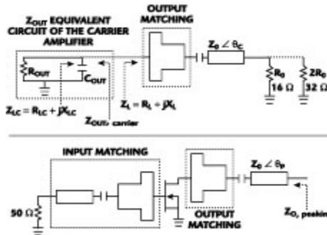
**Fig. 4** Load matching techniques to determine the angle of the offset transmission line for the (a) carrier and amplifier and (b) peaking amplifier.
