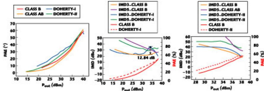
**Fig. 8** Power-added efficiency for the Doherty-I, Doherty-II, class B and class AB amplifiers vs. output power for a single-tone, 1.4 GHz signal.
