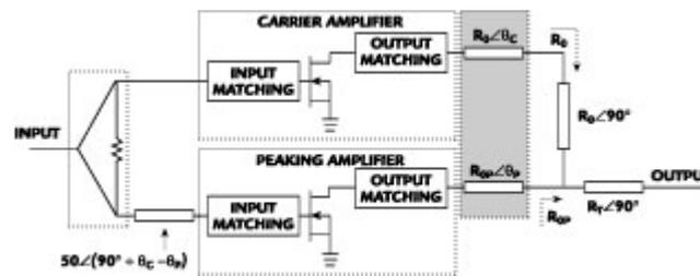
**Fig. 3** Schematic diagram of the proposed Doherty amplifier.
