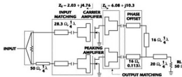
**Fig. 7** Implemented circuit diagram for a 1.4 GHz Doherty amplifier using Si LDMOS FET.
