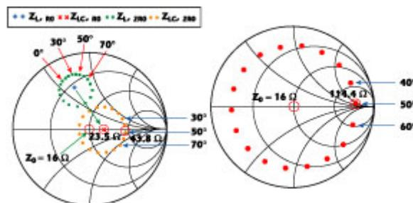
**Fig. 5** Simulated results for the load and **Fig. 6** Simulated compensated load output impedance of impedances for the carrier amplifier. output impedance of the peaking amplifier.
